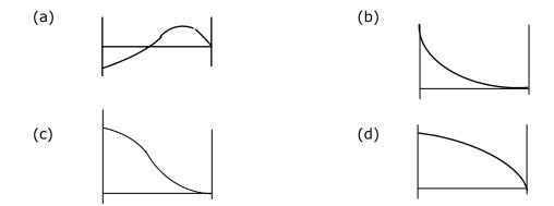
46. A cantilever beam has the square cross section of 10 mm $\times$  10 mm. It carries a transverse load of 10 N. considering only the bottom fibres of the beam, the correct representation of the longitudinal variation of the bending stress is
