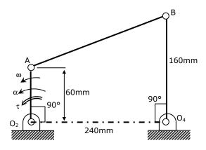
76. Which kind of 4-bar mechanism is  $O_2ABO_4$ ?
